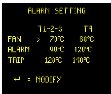
This menu shows the temperature set point for fan, alarm and tripping. The settings are common to the probes P1, P2 and P3, while P4 probe has a setting dedicated. By pressing the keys ↑ and ↓ you place the cursor on the desired set point; the key ← leads to a submenu that lets you change its value. After changing the value, press the button ← again to save the change or press the key MENU to return without the change.
