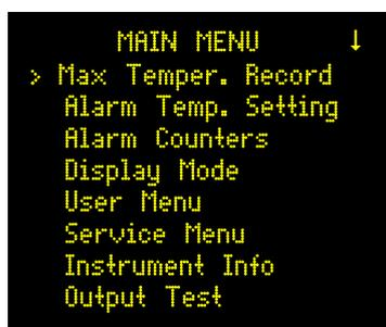
With the keys ↑ and ↓ you place the control on the desired line, with the key ← you access the submenu. When you are inside a menu, press the MENU button to exit and return to the main display.
